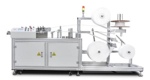
Automatic system to form 3 ply flat mask bodies, combine raw fabrics, three layers of pp non-woven, then form the creases, inserting nose clips and being weld together by ultrasonic welding device, finally cut into mask body pieces for next earloops welding procedure.
