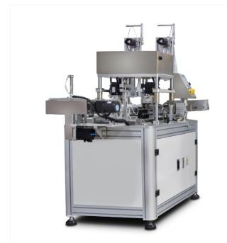
Used to weld the earloop on the mask bodies produced in previous process, featuring in fully synchronize with the tm120, no labors needed in the whole production process.
