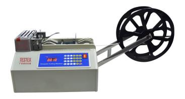
The rolled earloops are automatically cut into a specific length (18cm for adults) for the earloop welding process.
