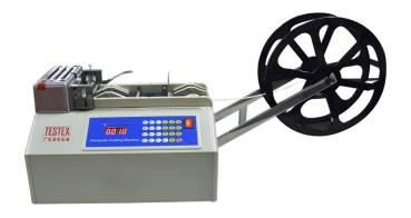
The rolled earloops are automatically cut into a specific length (18cm for adults) for the earloop welding process.
