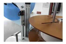
Add the nose wire shortage detection function to the alert system (previous model only have the detection on the shortage of mask fabrics), when the nose bridge is used up to avoid the production of masks with missing nose bridge.
