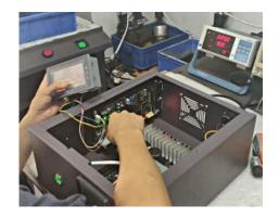
Each generator will perform repeated wave overload tests under the condition of 3 times the load of the simulated normal production parameters, so that the equipment can be started normally under any high-load work and the components will not be damaged.
