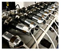
Each transducer will strictly detect core parameters such as resonance frequency, impedance and capacitance through professional instruments.
