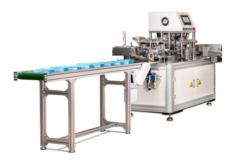
Fully integrated with mask bodies making machine, will sense the mask body delivered from the mask body forming machine, then fetch and weld the one set of earloop on each mask body, after the earloop being fold inwards, the mask pcs will be distributed to the auto packing machine (if ordered).
