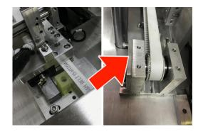
APL110 redesigned the position of the earloop fetching belt transmission structure, and changed the side transmission to the middle transmission. The uniform force makes a single belt have a longer service life and reduces the frequency and time of replacement of wearing parts.
